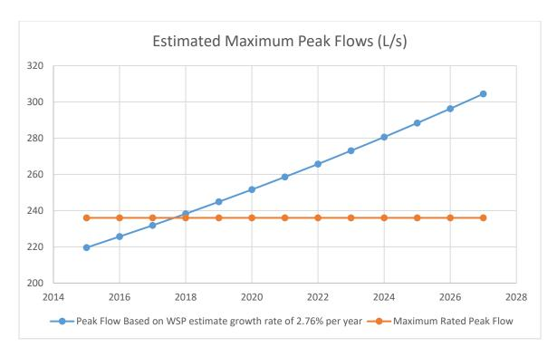
Figure 2-5: Estimated Maximum Peak Flows at Plant Over Time
