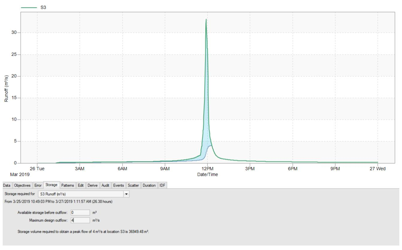
Hydrograph curve generated from the computer software PCSWMM approximating storage volume requirements for Subcatchment S3 during a 24 hour 100-year SCS Type II design storm.
