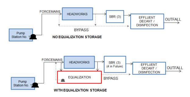
Figure 2-1: Potential Equalization Storage Below Headworks Building
