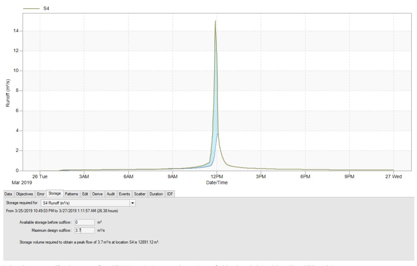
Hydrograph curve generated from the computer software PCSWMM approximating storage volume requirements for Subcatchment S4 during a 24 hour 100-year SCS Type II design storm.
