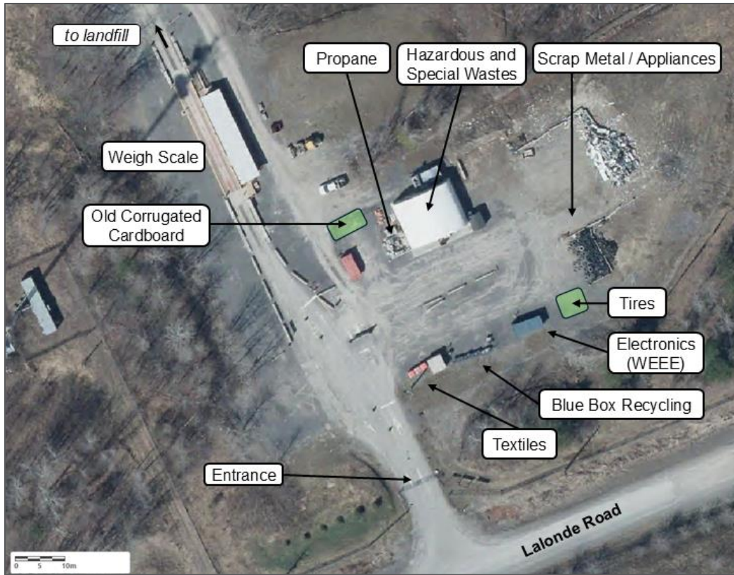
Figure 2: Scale House and Waste Diversion Drop-off Area
